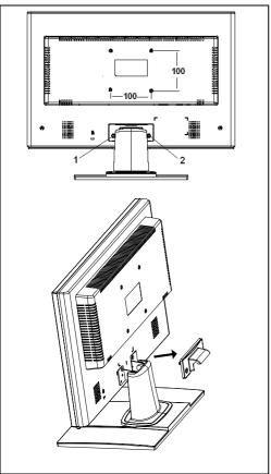
Remove the screws on the rear of the monitor
